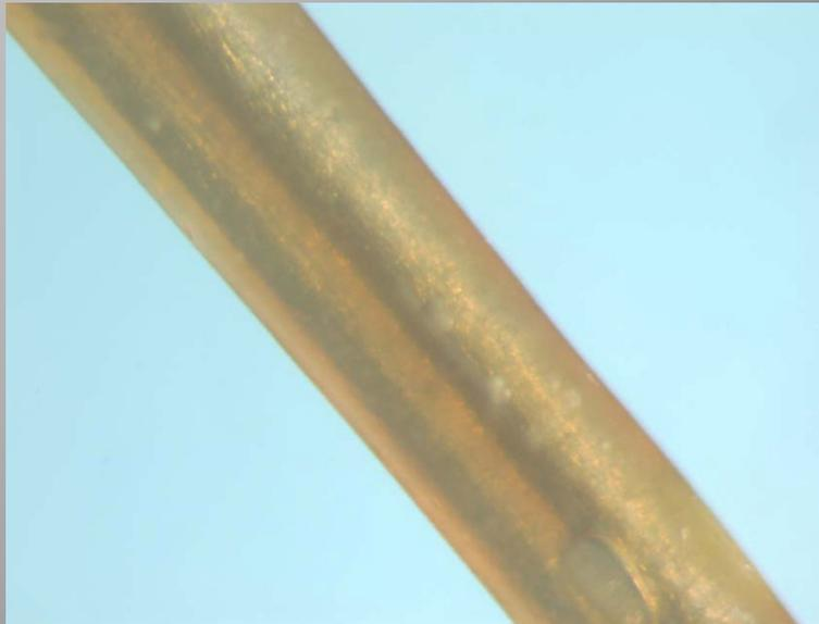
Titanium core, Dyed Titania, electrolyte counter electrode wire, photopolymer cladding
